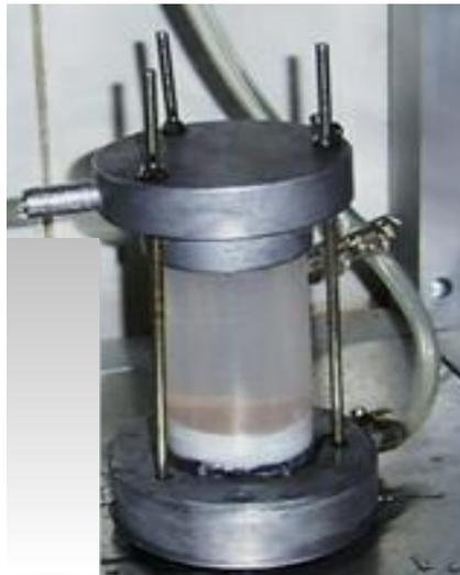
**Fig. 3:** General view of hydraulic conductivity test equipment[5]
